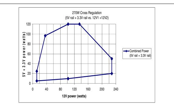
Figure 5 Cross Loading Graph for 270W Configuration
